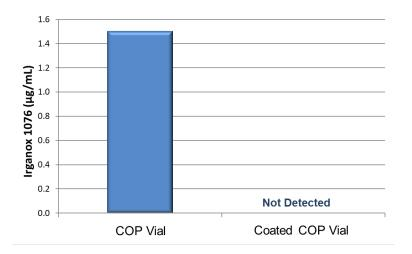
Figure B. Irganox 1076 extractables on uncoated COP and coated COP vials.
