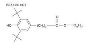
Figure A. Structure of Irganox 1076
